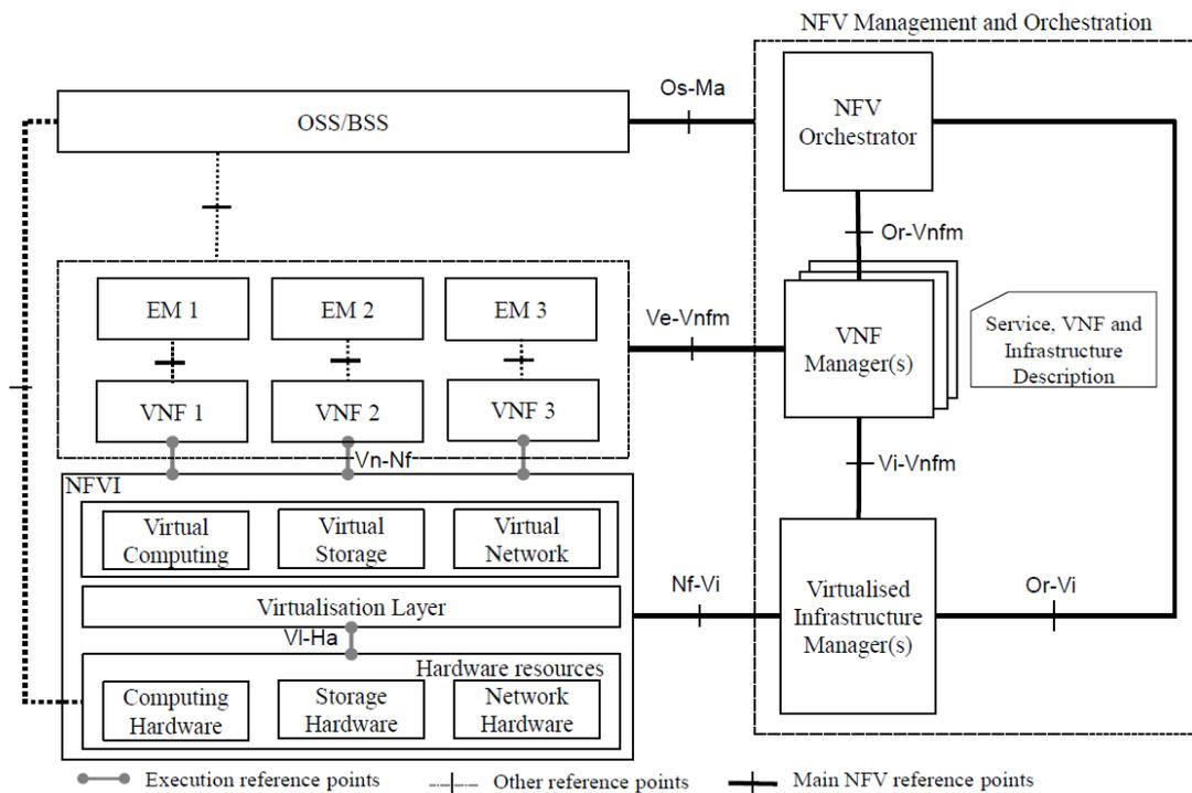
Fig 12.3-1: NFV reference architectural framework [ETSI ISG NFV]
