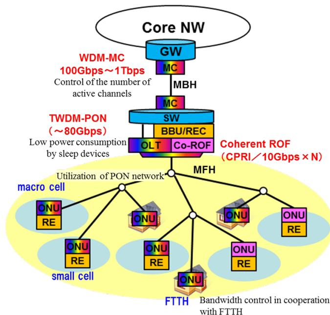
Fig. 12.4-8 Configuration of virtualized MFH/MBH using WDM technologies
