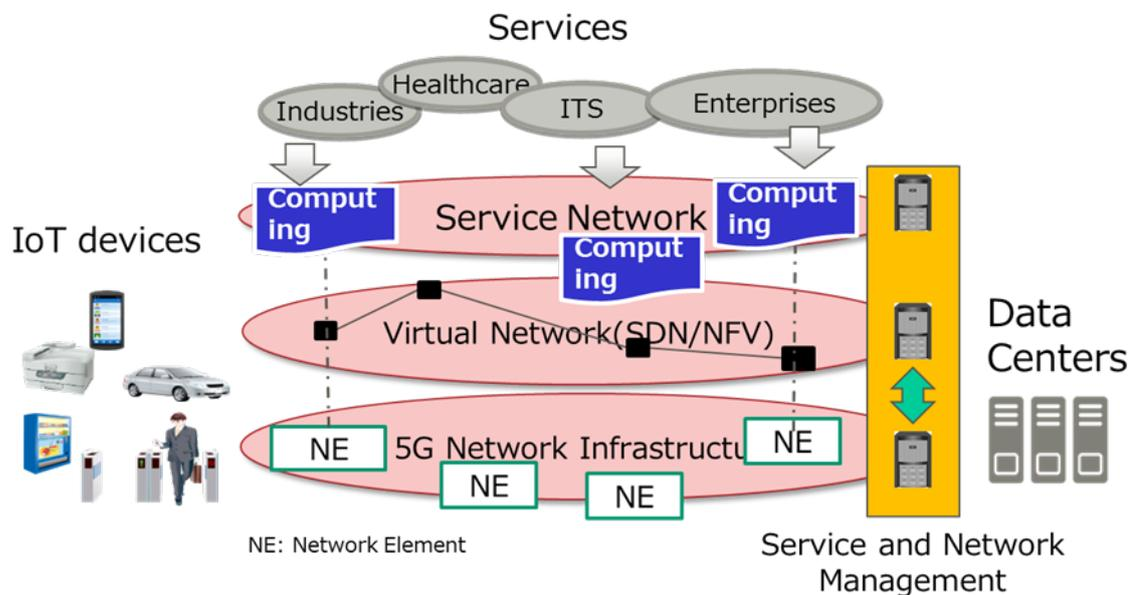
Fig. 12.3-8. The overview of Application-driven network configuration management.
