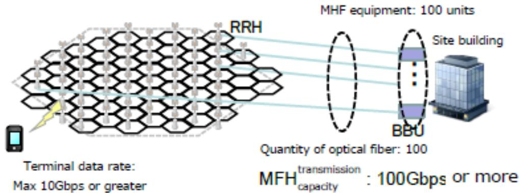
Fig. 12.4-4 Number of links at small cell
