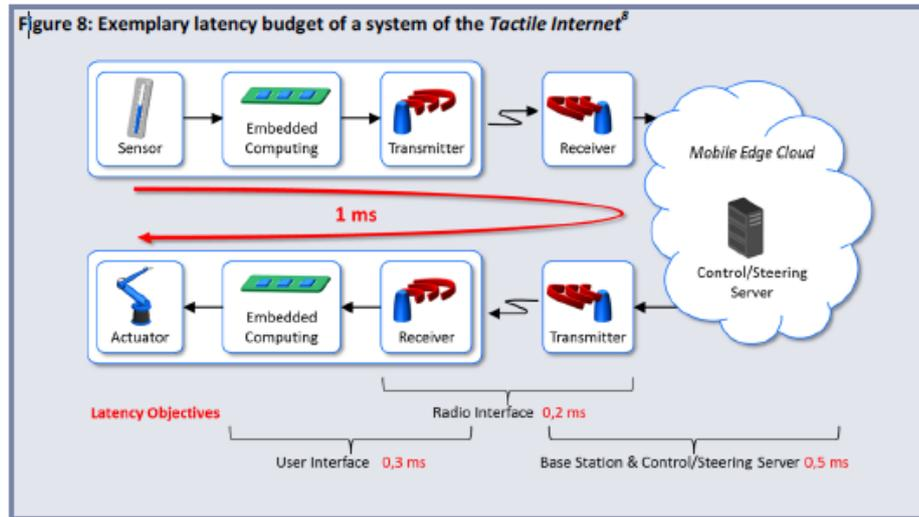
Fig. 12.5-5: Exemplary latency budget of a system of the Tactile Internet
