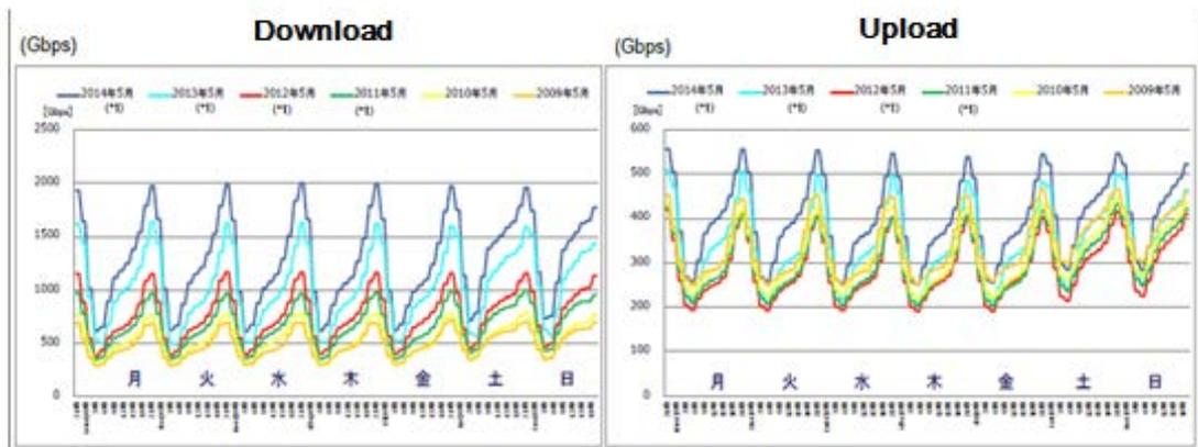
Fig. 12.3-2 Traffic fluctuation of Internet user data in Japan [MIC]
