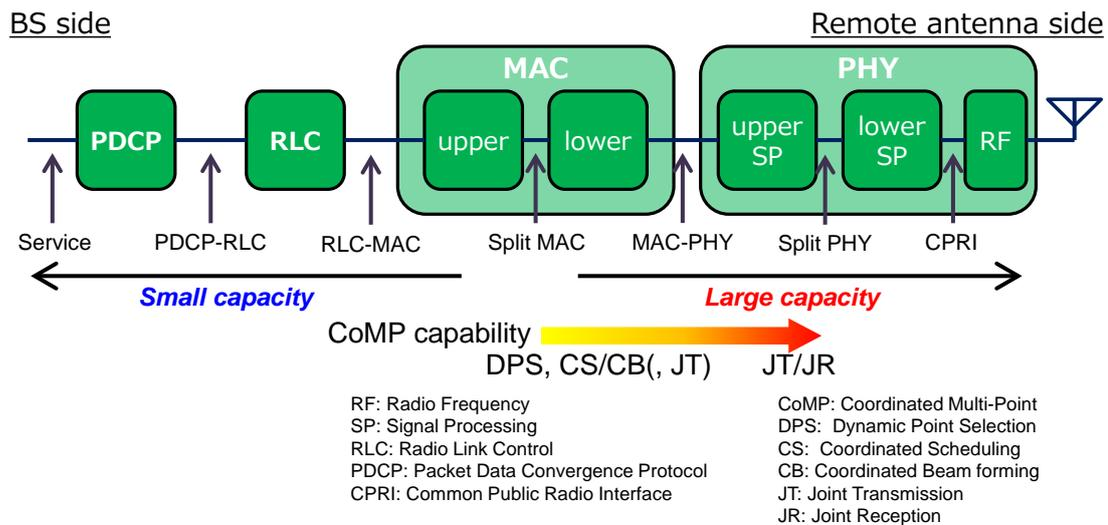
Fig. 12.4-9 Options of function split and required capacity
