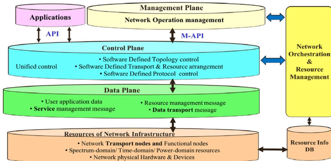
Fig. 12.3-6. Flexible mobile network – a logical structure
