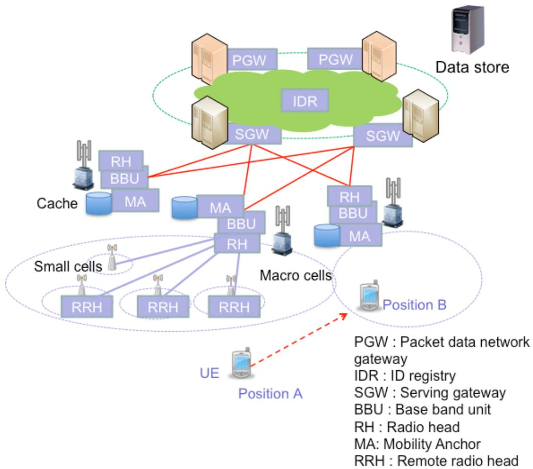
Fig. 12.5-10 – Distributed mobility anchor points and caching provisioning in 5G systems
