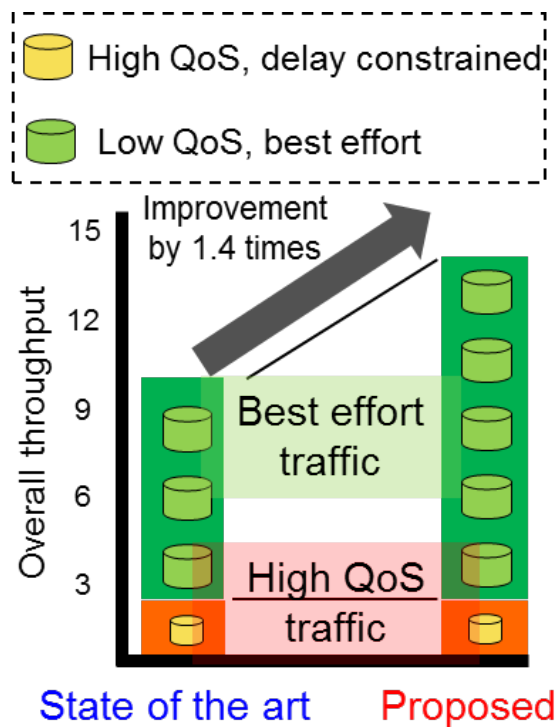
Fig. 11.3-13 A comparison of throughput gain, 70kbps assumed for delayed constrained high QoS applications, number of terminals for delay constrained and best effort applications is assumed to be 30 each
