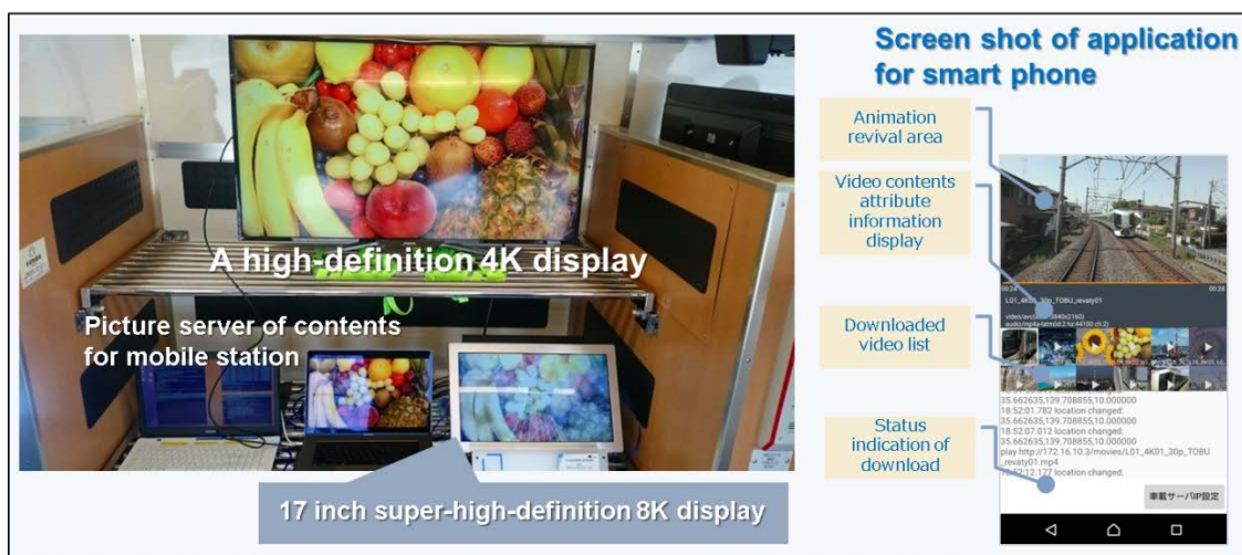
Fig.3.3.7 High-quality video delivery service for high-speed moving vehicles
