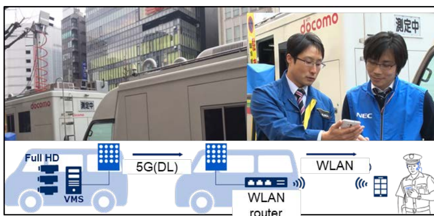
Fig. 3.2.5 Remote monitoring by high-resolution video for security
