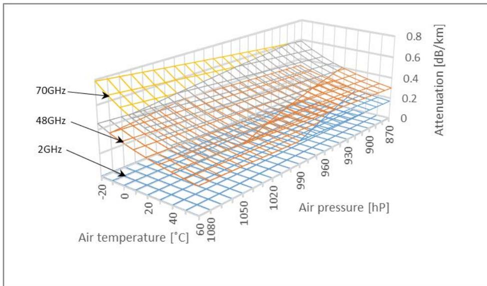
(a) Attenuation due to atmospheric gasses (vs. air pressure and temperature)
