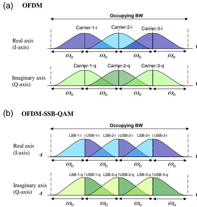
Fig. 11.3-1 Spectral structure of OFDM and OFDM-SSB-QAM
