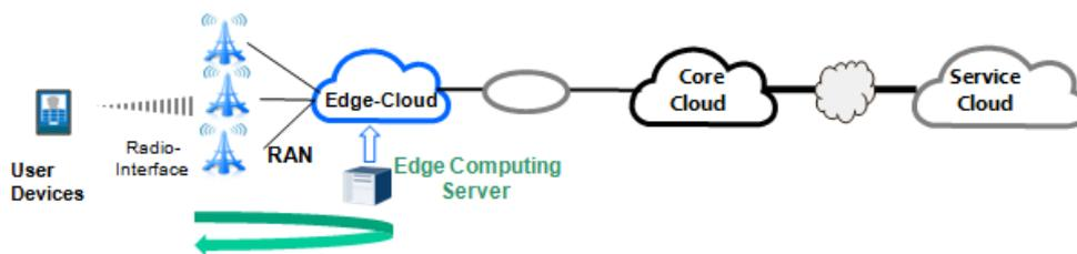
Fig. 12.5-6 Edge computing model for ultra-low latency networking
