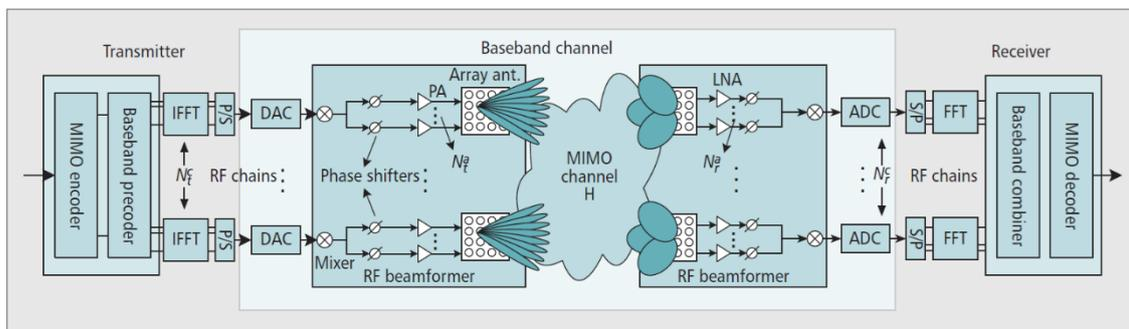
Figure 2. Block diagram of a hybrid beamforming architecture.
