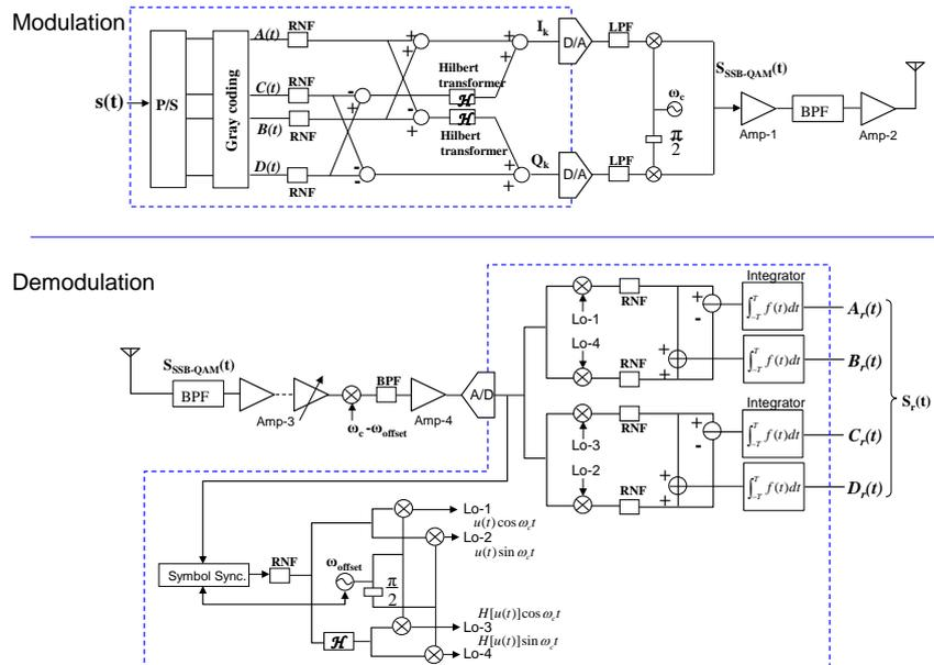
Fig. 11.3-2 Architecture of OFDM-SSB-QAM modulator and demodulator
