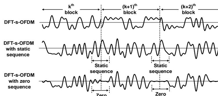
Fig. 11.3-3 DFT-s-OFDM with zero or static sequence insertion
