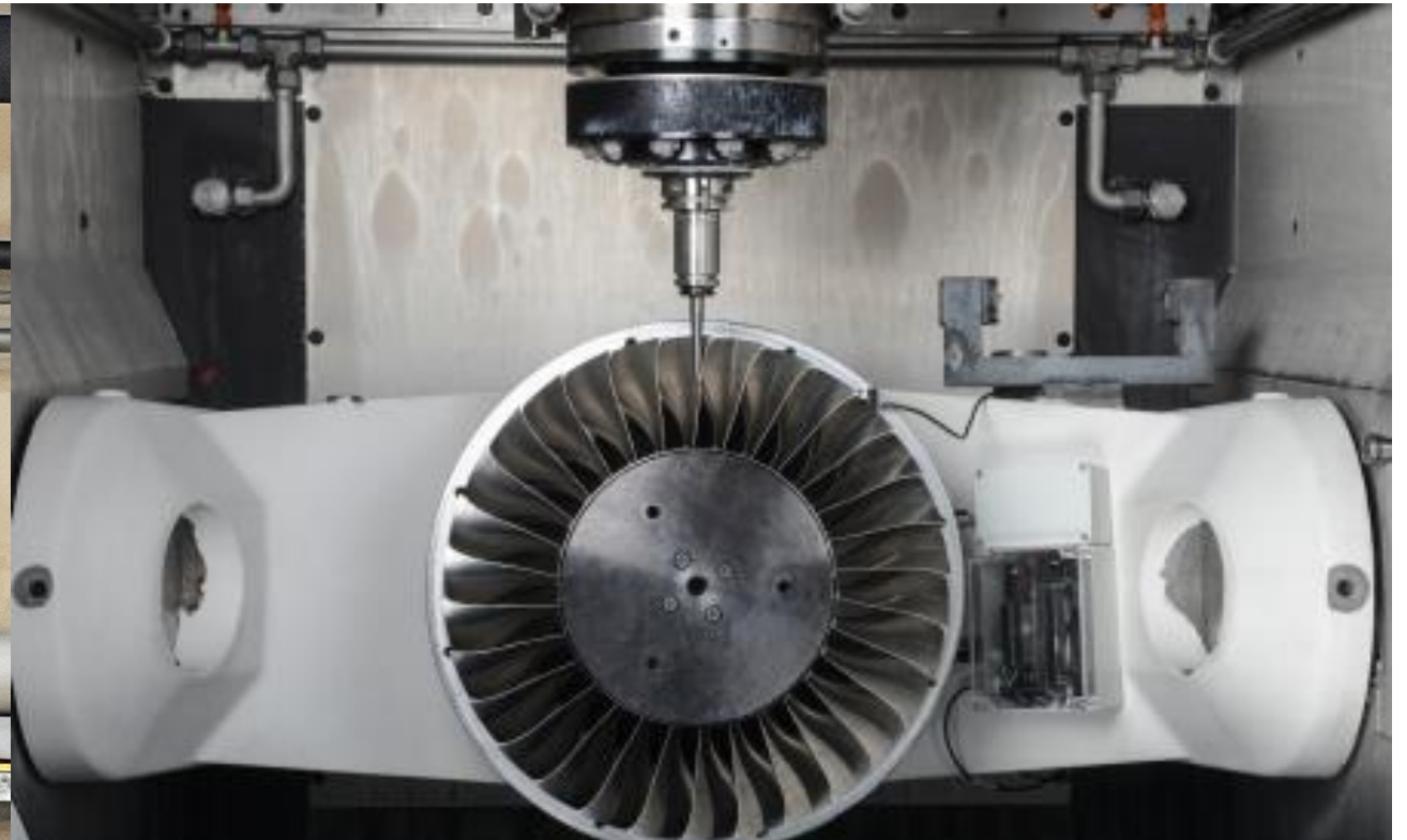
5G vibration sensor inside 5-axis milling machine
