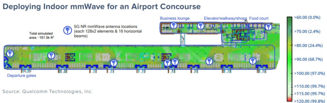
Fig. 5-5 Installation example of 5G millimeter wave base stations at airports and its measurement result [1]
