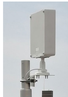
Fig. 9-9 Millimeter Wave Repeater (by DX Antenna)
